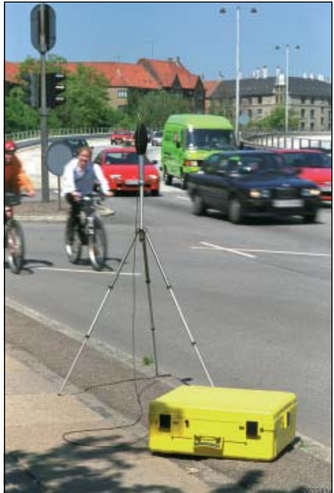
2260 Outdoor Gear measuring traffic noise on a busy urban road
